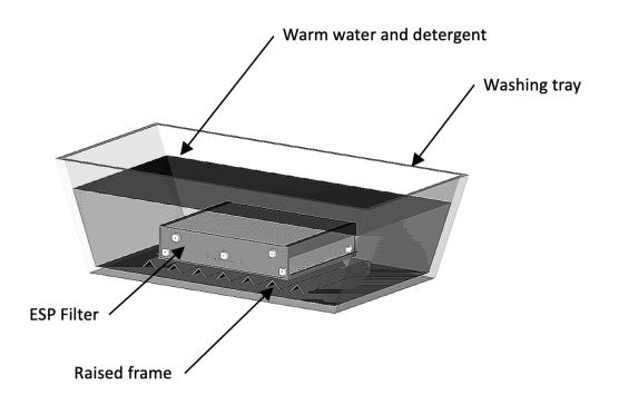
2. Remove the electrostatic cell and rinse thoroughly with running water, taking care not to break the ionisation wires.
